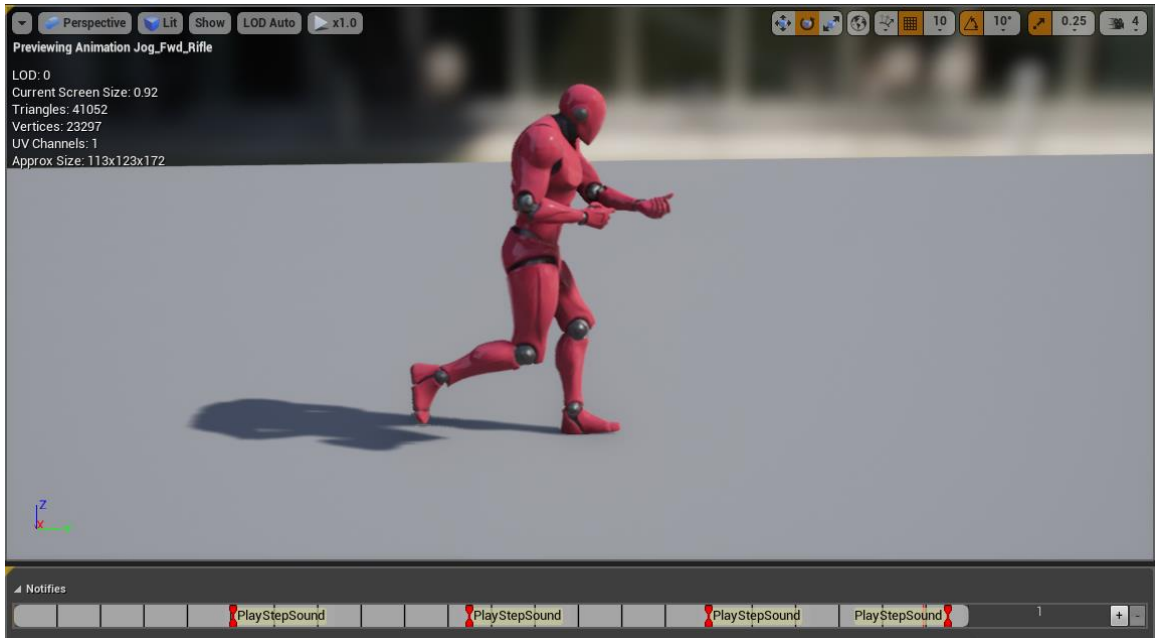
Figure 6: Assigning the function PlayStepSound whenever either of ML NPC's or BT NPC's feet hit the ground.
