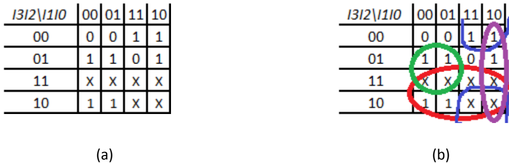
Figure 2.38: Segment g of the BCD to 7-segment decoder: (a) Original Karnaugh map; (b) One possible final Karnaugh map with prime implicants shown.
